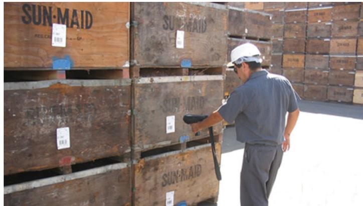
sorted, processed and packaged in cartons, boxes or bags with Global Trade Item Numbers (GTINs). The GTINs, encoded in bar codes, uniquely identify each item. The individual items are packed together in cases with ITF-14 bar codes and on pallets with GS1-compliant license plate bar codes.
